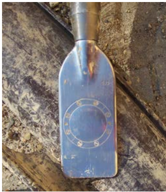
Fig. 4. Dilatometer blade after retrieval from borehole of stiff loess.
